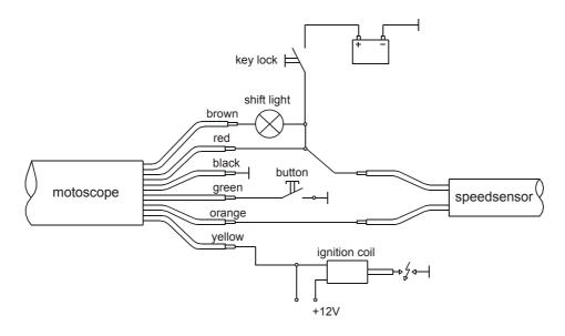
Remark: the gear shift light exit works only with the corresponding equipment with the correct poling. Our LED gear shift light has the following poling: core lead = plus, shielding = minus
